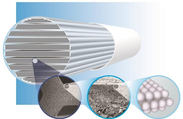
Feed channels are designed to maximize membrane surface area, while not compromising on flowrate. The unique surface coating and overall microstructure provide consistent, reliable removal of solids down to 30 nm in size.
